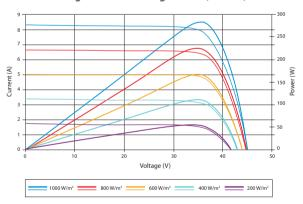
Exellent performance under weak light conditions: at an irradiation intensity of  $200\,\text{W/m}^2$  (AM 1.5, 25 °C), 95.5% or higher of the STC efficiency (1000 W/m²) is achieved
